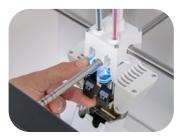
AA+ and CC+ print cores Quick-swappable nozzles that enable higher flow rate.
